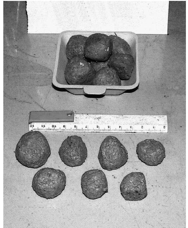
Fig. 8. An image of selected granules produced along the experimentation showing diameters up to about 30 mm.
